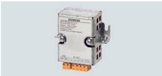
The Safe Brake Relay allows the Power Module to be safely connected to an electromechanical motor brake, allowing the brake to be directly and safely controlled by the Control Unit in accordance with EN 954-1, safety category 3, and IEC 61508 SIL 2.
