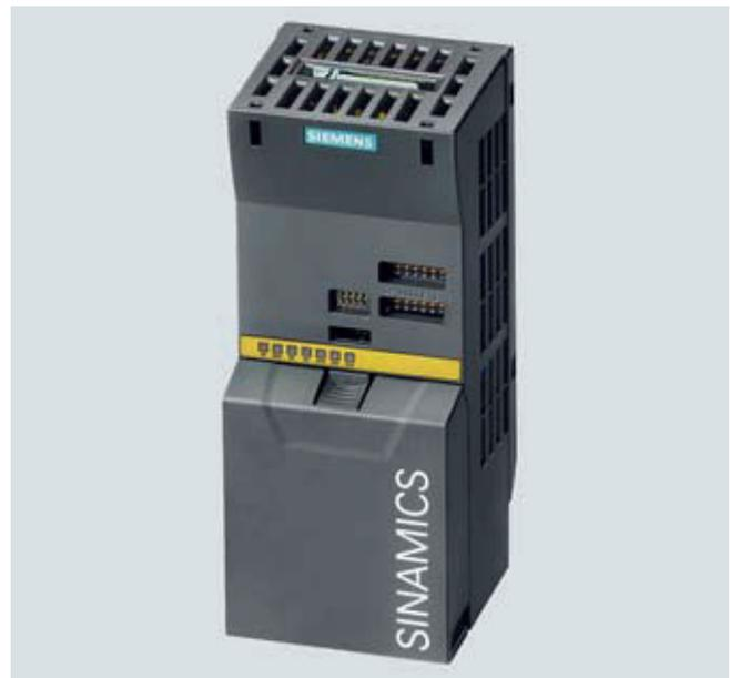
Control Unit with inserted MMC memory card
