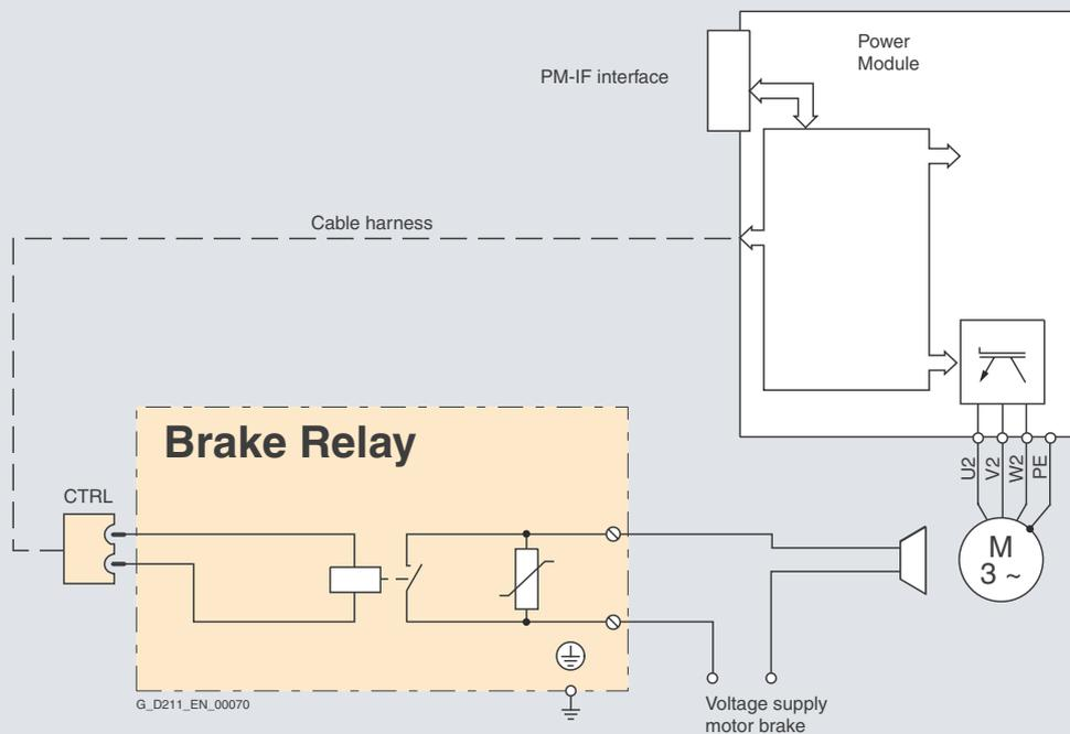
Connection example for Brake Relay
