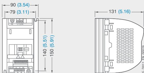
Inverter frame size FSA; 0.55 kW (0.75 hp) to 0.75 kW (1.0 hp)
