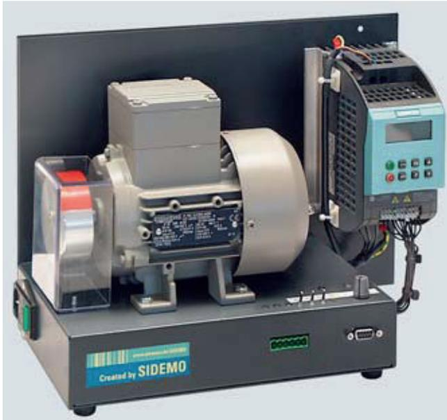
The modular SIDEMO case system for micro-systems also includes a training case for SINAMICS G110 which is designed for mobile use for sales and servicing.
