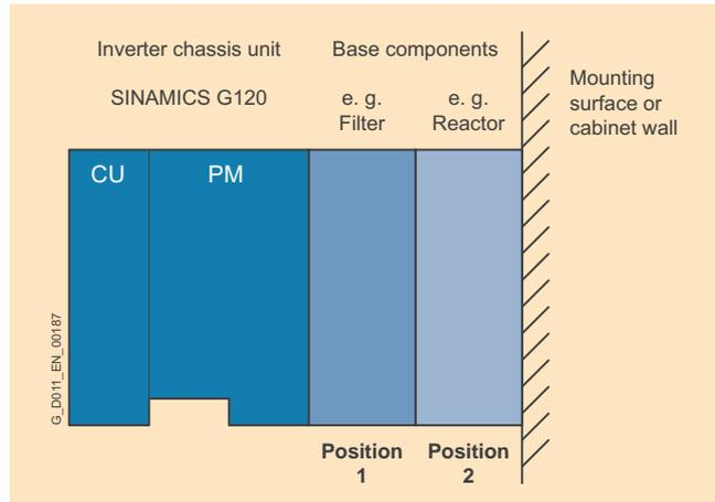
Frequency converters, consisting of Power Module (PM) and Control Unit (CU) and two base components at positions 1 and 2
