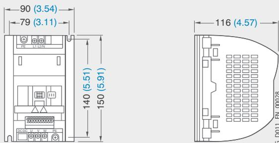
Inverter frame size FSA; 0.12 kW (0.16 hp) to 0.37 kW (0.5 hp)
