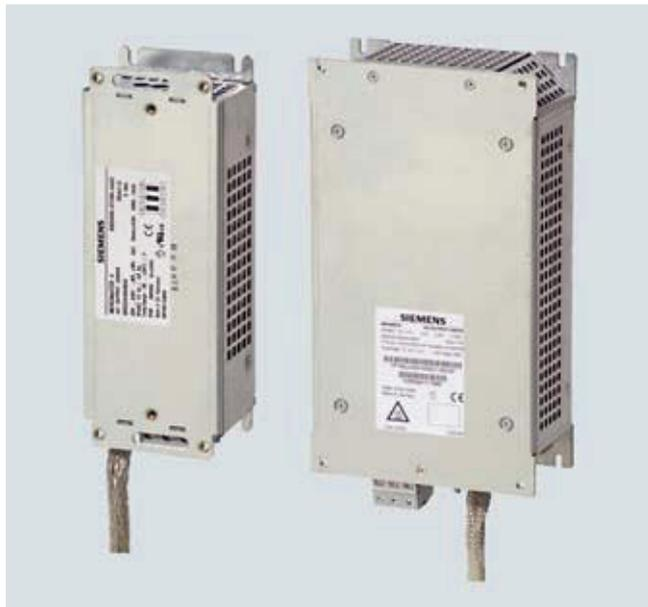
Output reactors reduce the voltage loading on the motor windings. At the same time, the capacitive charge/discharge currents, which place an additional load on the power section when long motor cables are used, are reduced.
