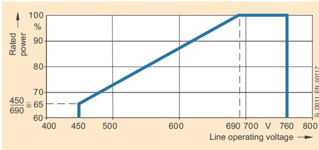
The power units can also be operated on a minimum voltage of 500 V –10%. In this case, the power is reduced linearly as required.
