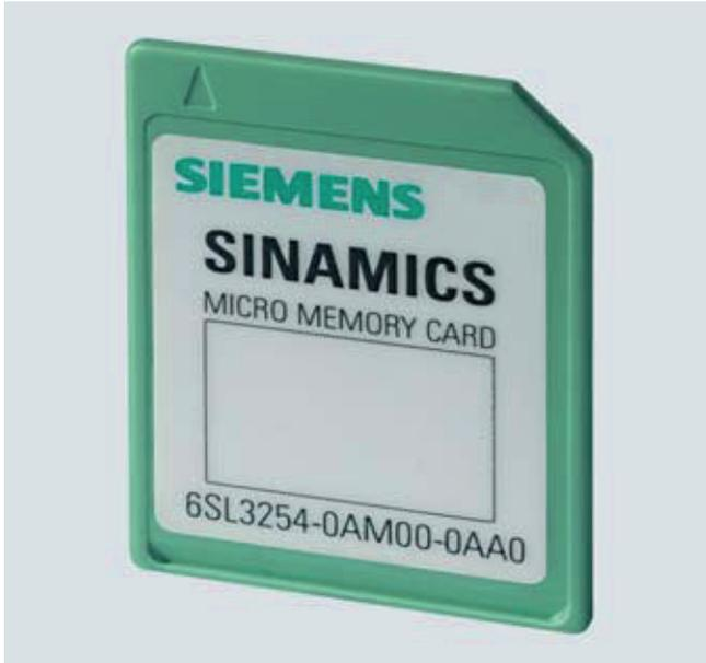
The parameter settings for an inverter can be stored on the MMC memory card. When the plant is serviced, it is immediately ready for use again after, for example, replacement of the frequency inverter and transfer of the memory card data.
