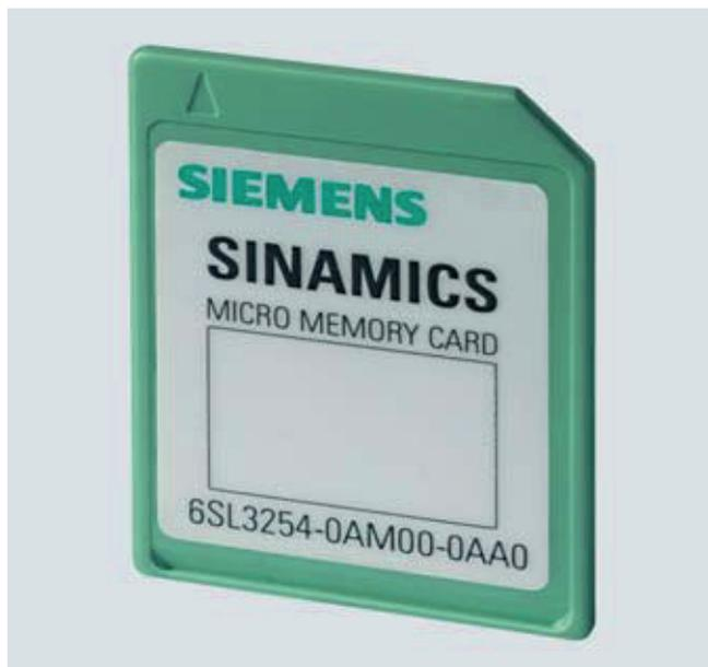
The parameter settings for an inverter can be stored on the MMC memory card. When the plant is serviced, it is immediately ready for use again after, for example, replacement of the frequency inverter and transfer of the memory card data. The associated slot is located on the rear of the Control Unit.
